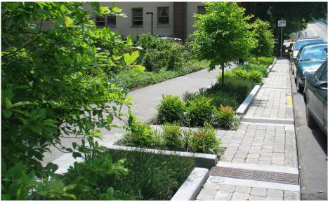
Image of a stormwater curb extension. Courtesy of Philadelphia Water Department.
